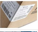
Corner wrap labels or dual tamp system can be used to apply information to adjacent sides of cartons
